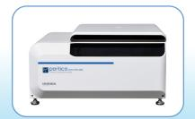
The **Partica CENTRIFUGE CN-300** applies centrifugal force of up to 30,000g and uses temperature control to produce accurate measurement results for a variety of samples. The key feature of centrifugation is that the particle size is measured following classifying by size, resulting in a very wide range of high-precision measurements.
